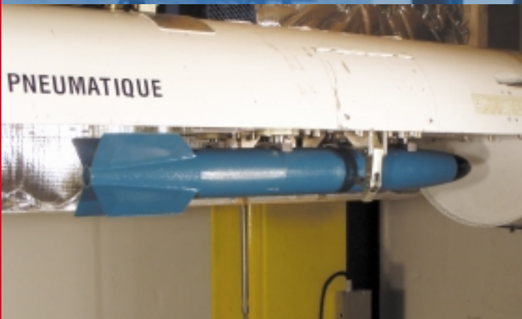
The Rafaut LBF2 Pneumatique ejector rack fitted with 14kg Practice Bombs
